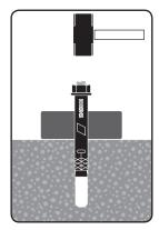
· Insert anchor into position.
