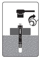
with correct size socket or spanner tighten anchor to specified torque
