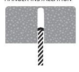
With the correct diameter drill bit, drill a hole to the correct depth (add at least one anchor diameter to the depth to prevent the fastener from bottoming out).
