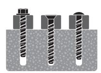
Continue to tighten the anchor until flanged head is firmly seated against fixture. Installation complete!
