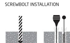
With the correct diameter drill bit, drill a hole to a depth of at least one anchor diameter deeper than required embedment.
