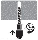
Attach the Anchor to the correct size socket driver and install anchor perpendicular to the base material substrate. Be sure not to over torque the anchor.
