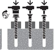
Install with either a socket or cordless impact driver. Apply pressure against the fixing and rotate to engage the first thread.
