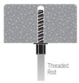
The head of the anchor should be set flush with the base material. Install the threaded rod. The thread should be fully engaged in the anchor.
