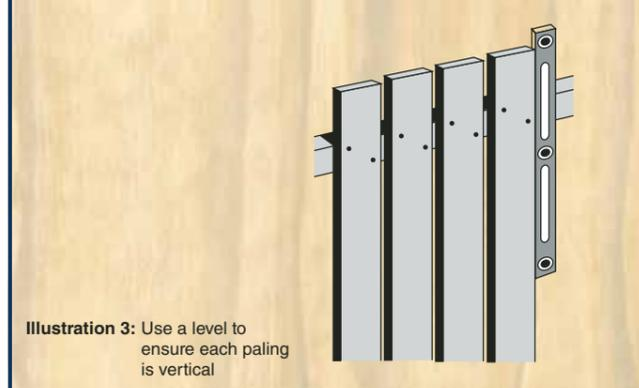
Illustration 3: Use a level to ensure each paling is vertical
